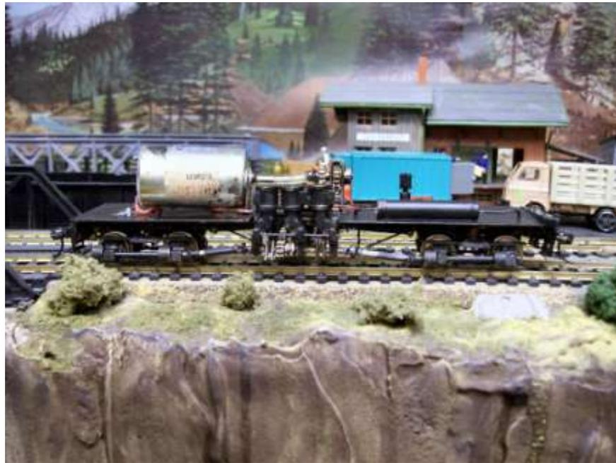
The superstructure was missing the front bolster and steps. I found a plastic one in the junk box and glued it on. Kadee couplers were added. A rear headlight was purchased from Custom Railway Supply. I still haven't done anything with the headlight or stack screen. Careful application of flat black from a 'rattle can' produced good results. I also painted the interior to eliminate brass shine. The locomotive was reassembled, and runs well. Shays are NOISY! Don't think I'll try to install DCC.
