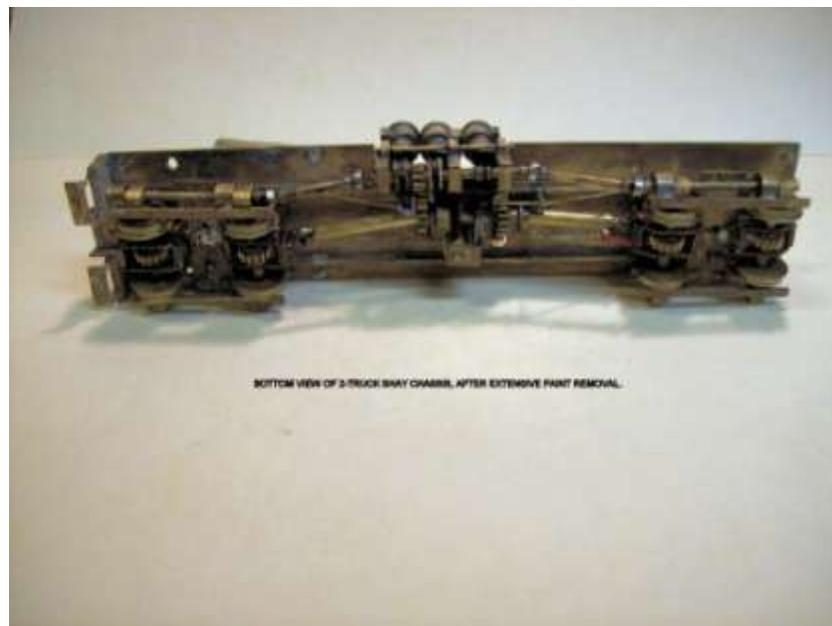
With the motor re-installed (It was a replacement can motor from Wayne Lemle's store sometime in the past, for \$17.95) I placed the chassis on the track and tried it out. Motor ran, mechanism tried to move, but jammed. Then the tubing started slipping on the drive gear. A shot of "super glue" stopped the slipping, but the mechanism still didn't want to turn. I banged on it some more.
